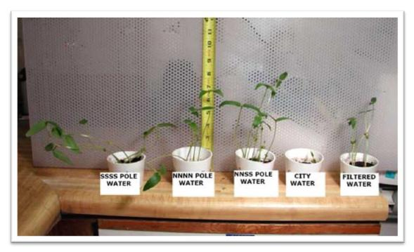
The three pots on the left were fed magnetized filtered water with varying magnetic configurations. The two pots on the right were fed non-magnetized water.
